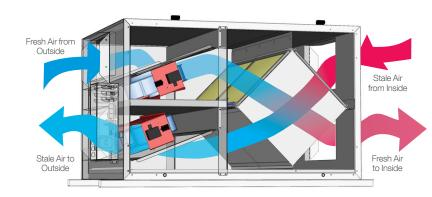
In the heating season, Heat Recovery Ventilators (HRV) and Energy Recovery Ventilators (ERV) draw in fresh air from outside while stale, humid air is exhausted. As the fresh and stale airstreams pass through the unit's core, the fresh air is tempered with heat recovered from the exhaust air. In the cooling season, fresh outdoor air is cooled by the air-conditioned exhaust air. An ERV will also transfer moisture to improve comfort in homes.
