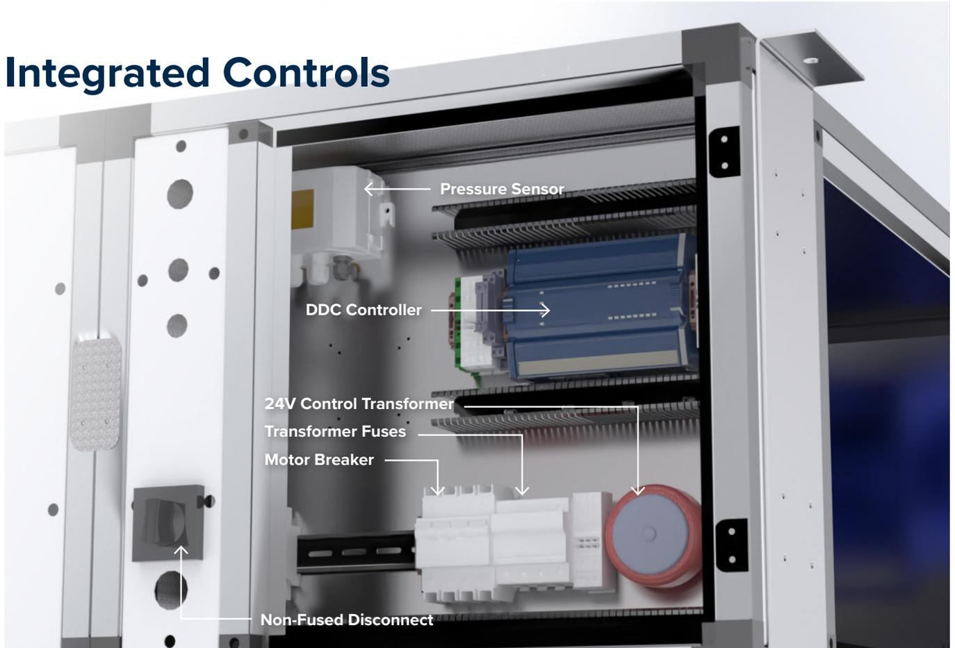
Terra features an integral control box, all control components come factory-installed.
