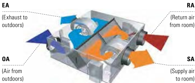
Heat exchanger with high temperature and enthalpy efficiency
