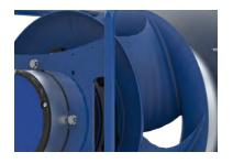
The plug fan has the impeller fitted with air foiled blades to obtain the highest possible efficiency. The fan is a single inlet, free-blowing fan where the unit casing acts as fan housing. The plug fan has a static efficiency of up to 75%. The plug fan can be supplied with EC motor (IE5), PM motor (IE4), or AC motor (IE3). Fan impeller and motor are statically and dynamically balanced.
