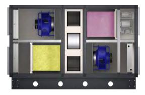
The heat pump is an integrated reversible heat pump system built into a unit section. The system consists of a reversible heat pump and a rotary heat exchanger that enables both heating and cooling. The unit is equipped with scroll compressors, and cooling/heating capacity is stepless variable in the range 5-100%. The heat pump is based on R-410A refrigerant. The heat pump is equipped with a complete control system.
