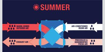
IN SUMMER, THE WARM, HUMID OUTSIDE AIR IS PRECOOLED AND DEHUMIDIFIED BY THE OUTGOING COOL INTERIOR AIR
